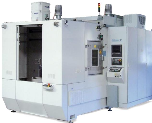
**VectorJet III** from PILLER Entgrattechnik: The high-pressure system has the same degree of freedom as a 4-axis machining centre and can be automatically loaded and unloaded.
